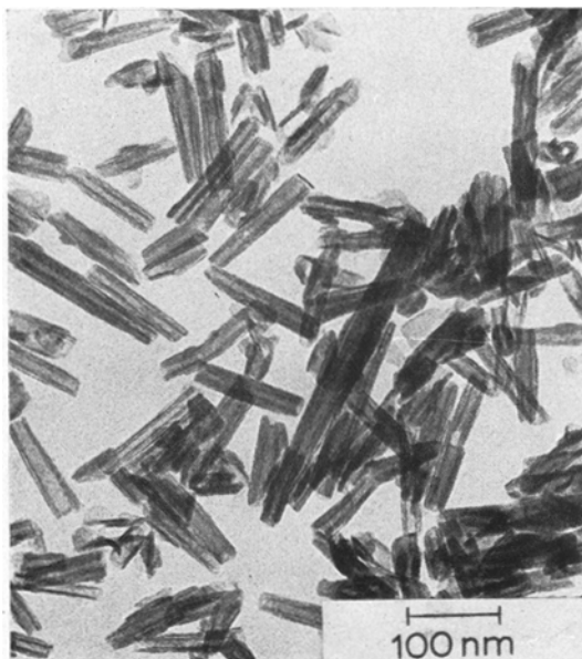
Figure 6 Electron micrograph of totally dehydrated synthetic garnierite. Maximum dehydration temperature: 600°C.
