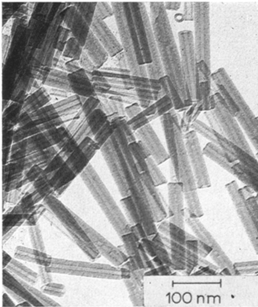
Figure 1 Electron micrograph of synthetic chrysotile.
